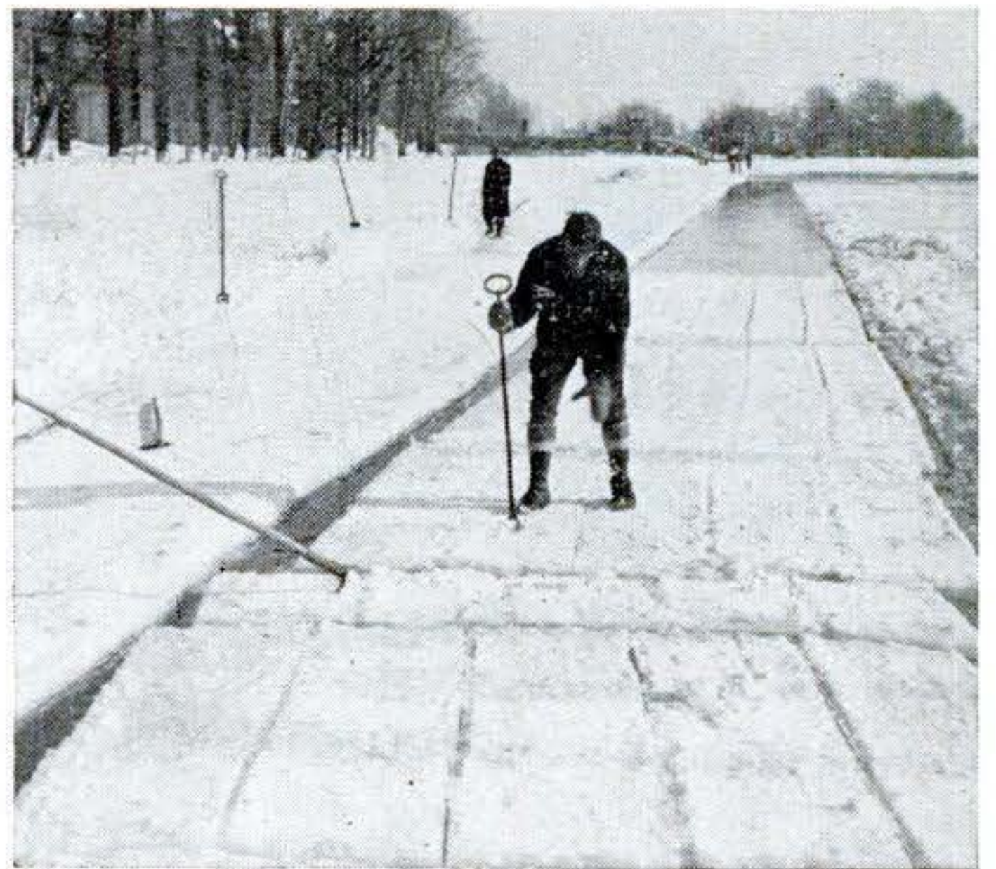
5. Floats of five cakes ride the channel. As these approach the conveyer, barring forks are used to split them through below the point reached by the saw, producing single cakes.
